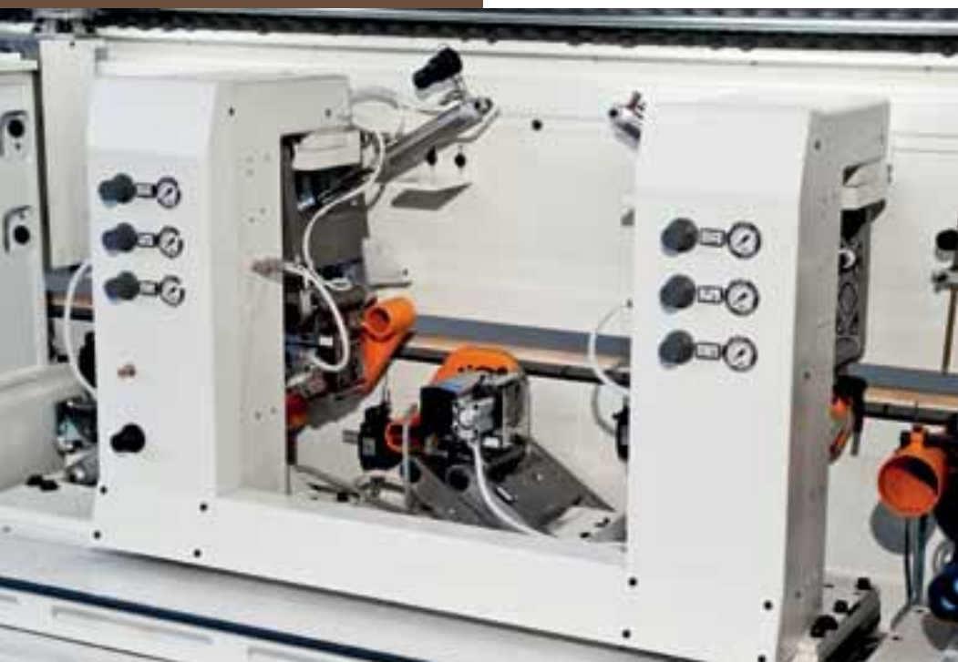
4 motors corner rounding unit
